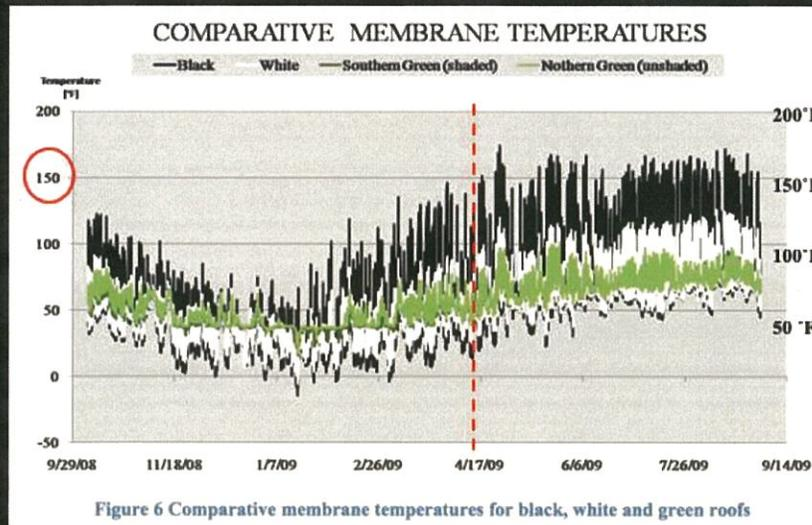
Figure 6 Comparative membrane temperatures for black, white and green roofs
