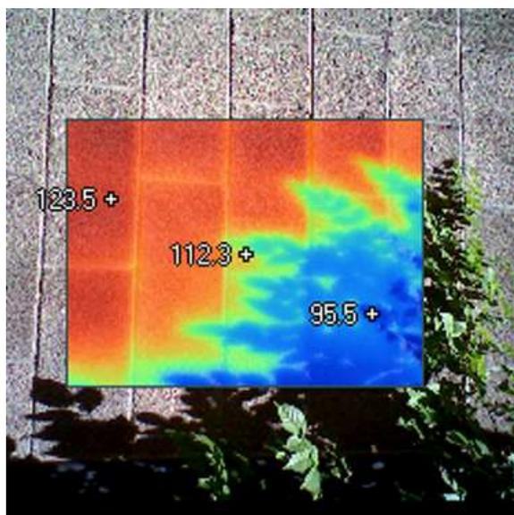
Infrared photo, superimposed on a masonry surface with green wall, shows difference in temperatures.
