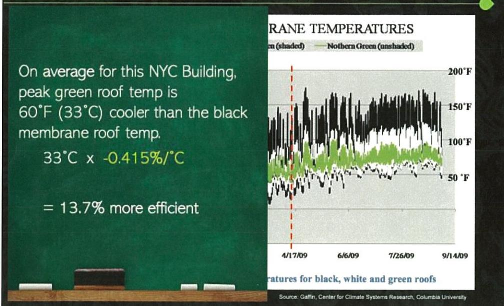
The black membrane reached a peak temperature of  $176^{\circ}\text{F}$  ( $80^{\circ}\text{C}$ ).
