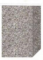
The two foot depth of glass aggregated on the right allow for the storage a 1' of flood waters per square foot of walkway, roadway, parking lot, or rain garden. This provides a way for Jamaica Bay communities to build their way out of future flooding threats, storing water for the growth of trees and meadow, treating water and cleaning air in the process,
