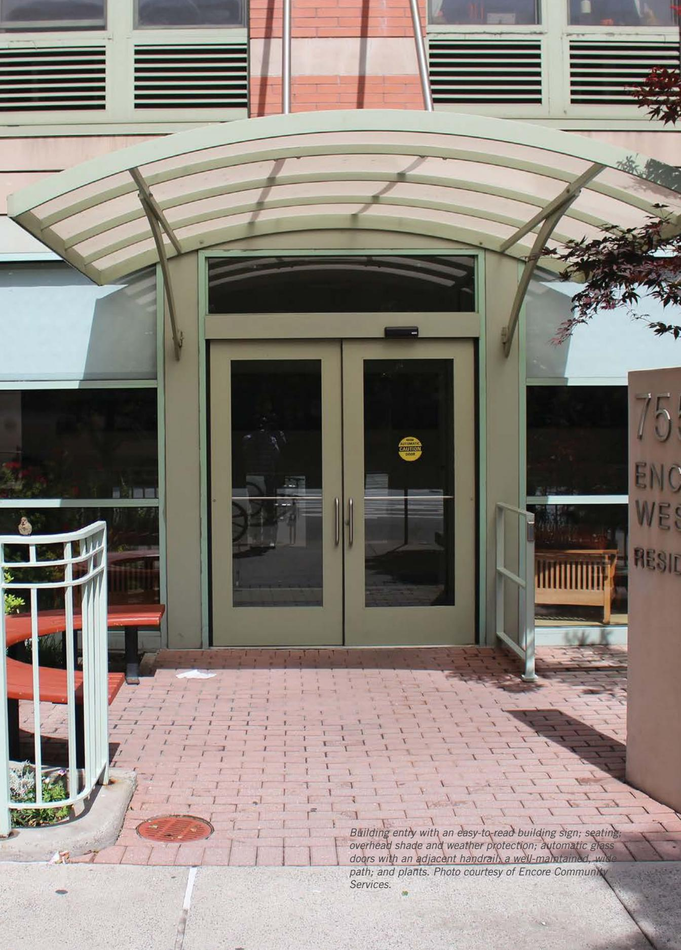
*Building entry with an easy-to-read building sign; seating; overhead shade and weather protection; automatic glass doors with an adjacent handrail, a well-maintained, wide path; and plants. Photo courtesy of Encore Community Services.*
