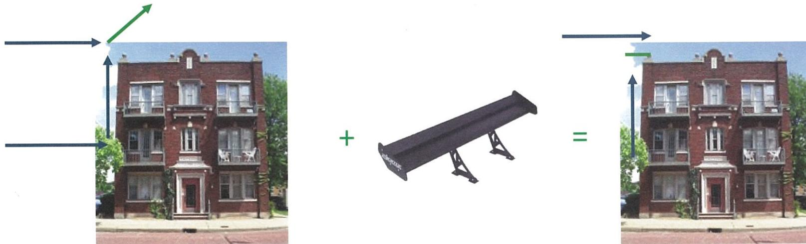
Use of spoiler and other roof aerodynamics enables less turbulent rooftop wind aimed at the turbine.
