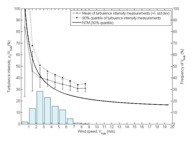
Figure 6. Turbulence intensity and wind distribution, 2 m above rooftop in Melville, Western Australia, during January-February 2009 (Whale, Ruin, and Tokuyama 2012)
