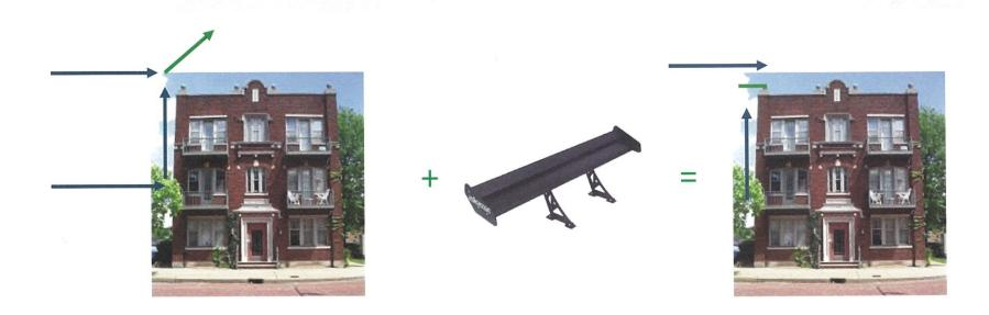
Use of spoiler and other roof aerodynamics enables less turbulent rooftop wind aimed at the turbine.
