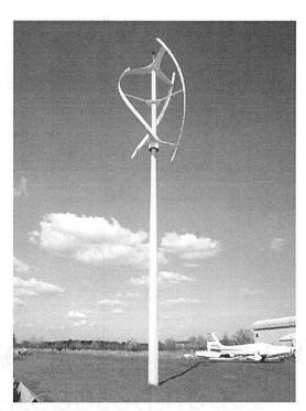
Example of a Vertical-Axis Wind Turbine
