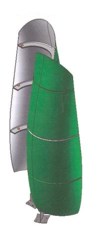
Turbulent areas are divided by horizontal ribs according to a specific formula
