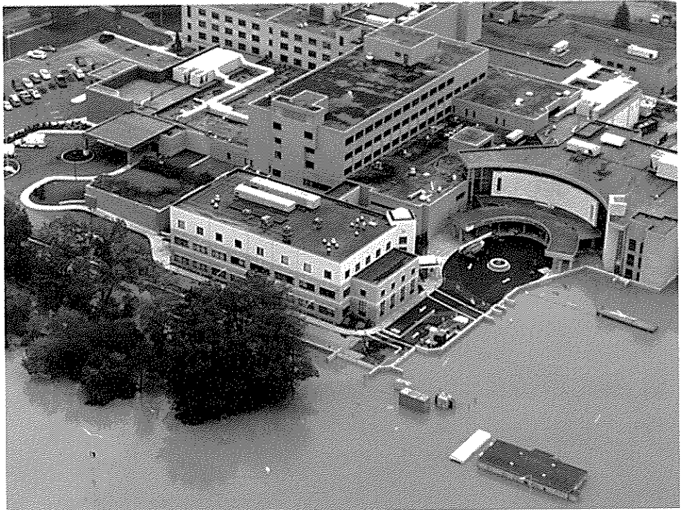
Hospital protected from flood water by a flood wall in mid-state New York. Photo credit: FEMA
