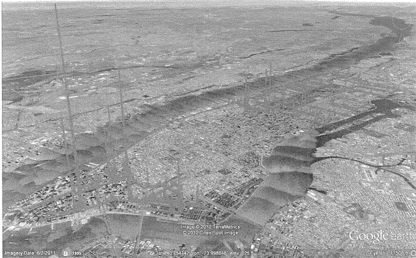
Image 2. Results of methane survey of parts of Manhattan on 28 November 2012
