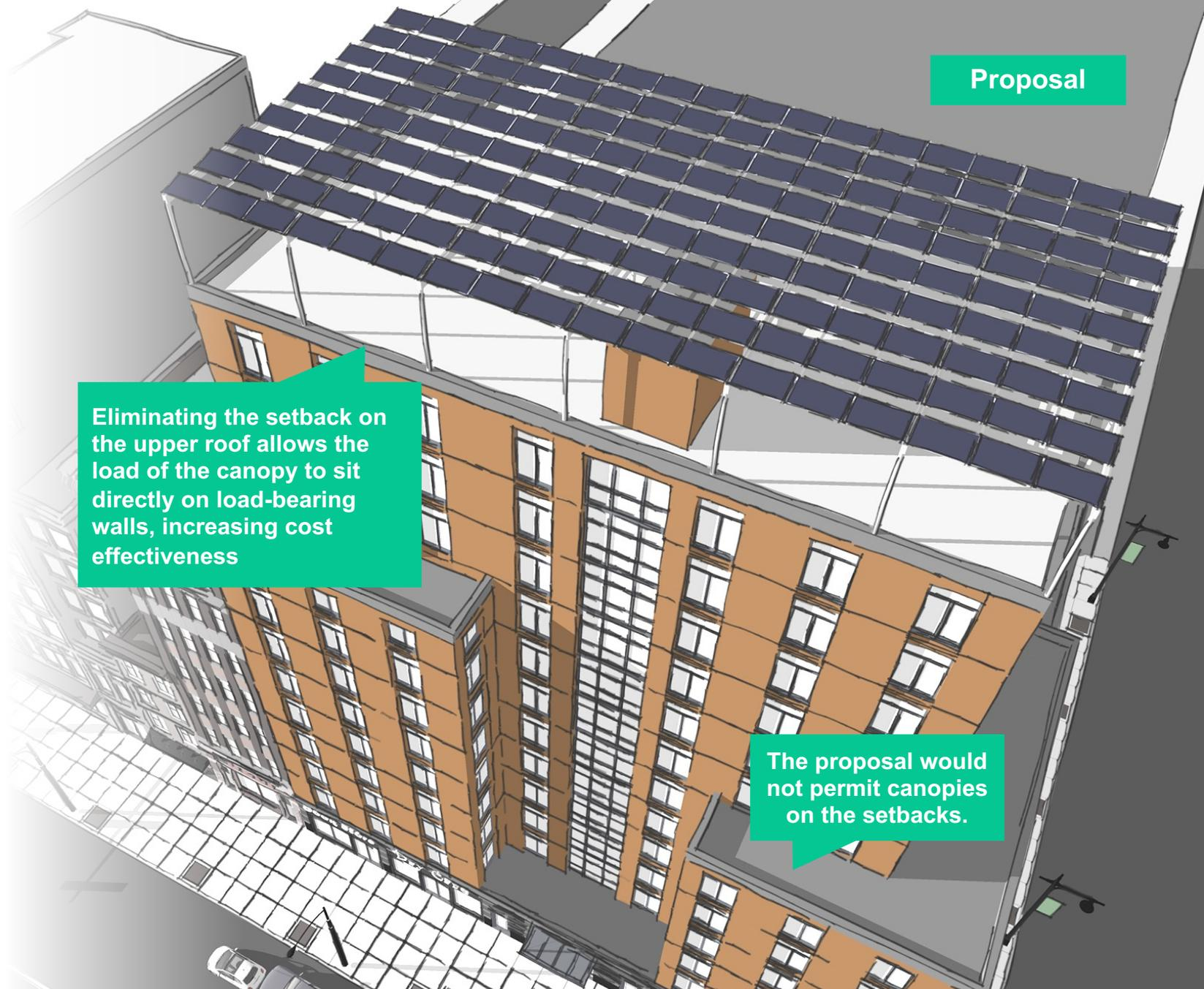
Eliminating the setback on the upper roof allows the load of the canopy to sit directly on load-bearing walls, increasing cost effectiveness
