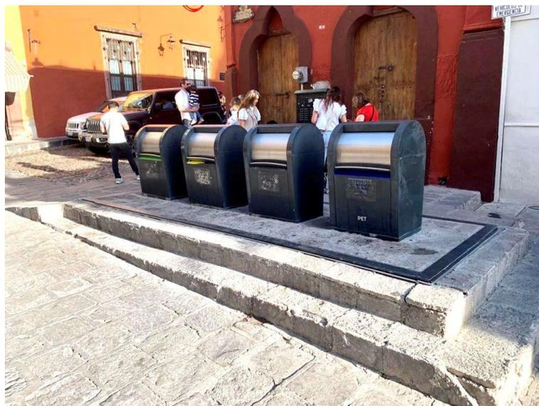
Buenos Aires, Argentina has bilateral collection systems that makes waste collection twice as fast while keeping the trash in an enclosed high-capacity container at all times. In none of these systems trash is collected by hand. They are collected by mechanical lifters, that make the collection faster, as well as safer for the worker.
