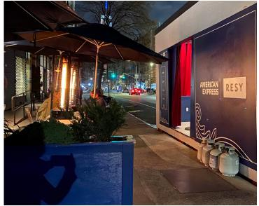
Improper propane tank storage; propane heaters too close to combustible materials
