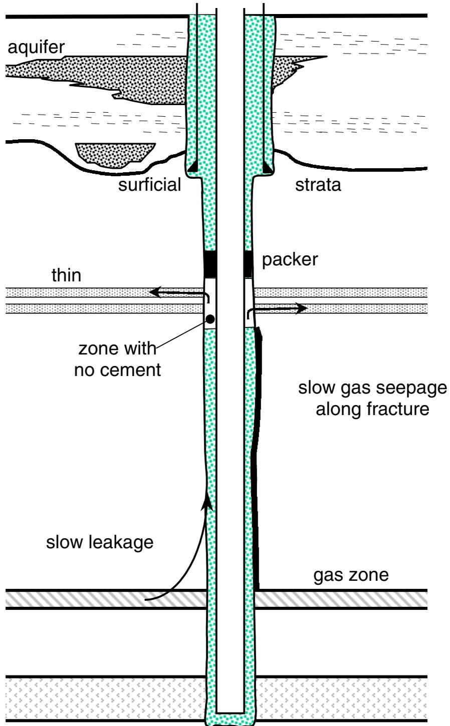
**Figure 5: Leaving a Leak Off Zone to Arrest Gas Seepage**
