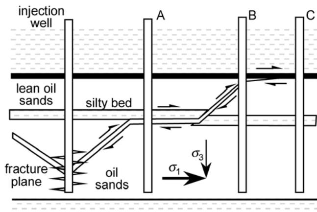
Fig. 16—Sequential fracture-induced casing shear.
