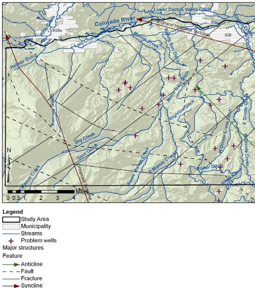
Figure 5. Location of gas wells with persistent or reoccurring bradenhead pressures greater than 100psi, from Albrecht (2007).
