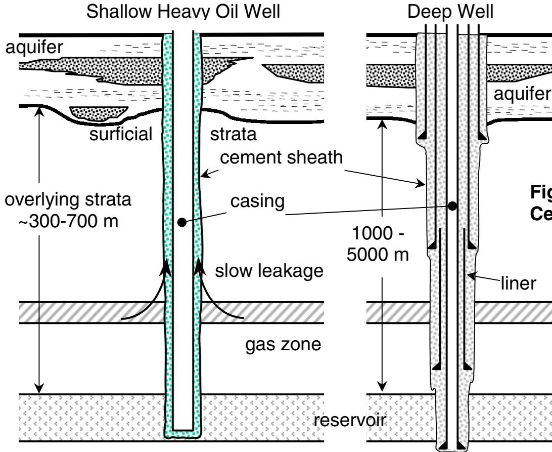
Figure 1: Cased, Cemented Wells
