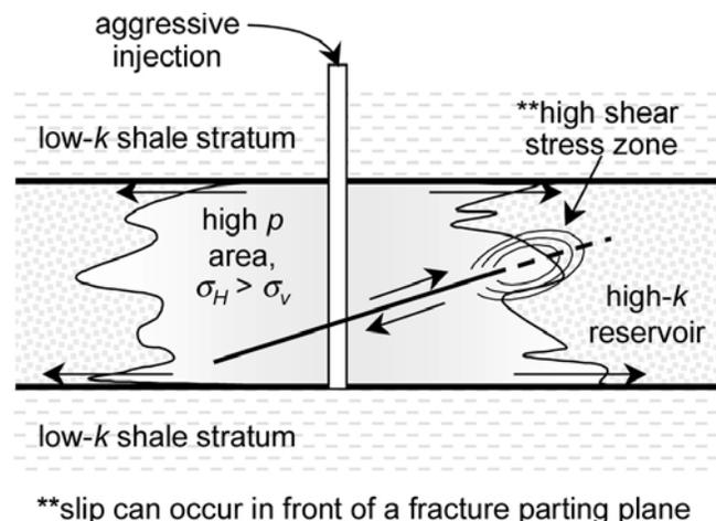
Fig. 7—Low-angle injection-induced shearing.
