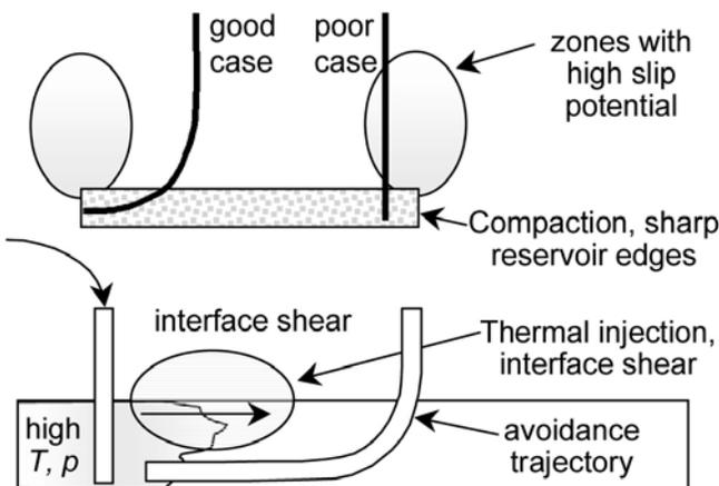
Fig. 18—Avoidance of zones of maximum slip.
