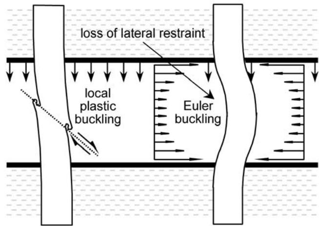
Fig. 11—Euler buckling and plastic buckling.
