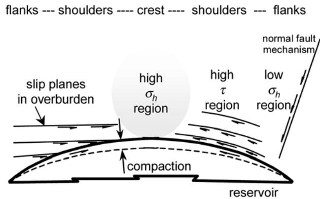
Fig. 5—Compacting reservoir bedding-plane slip.
