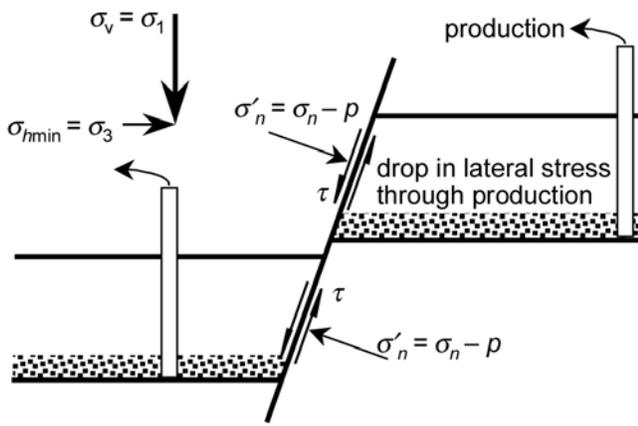
Fig. 8—Normal fault-triggering during production.
