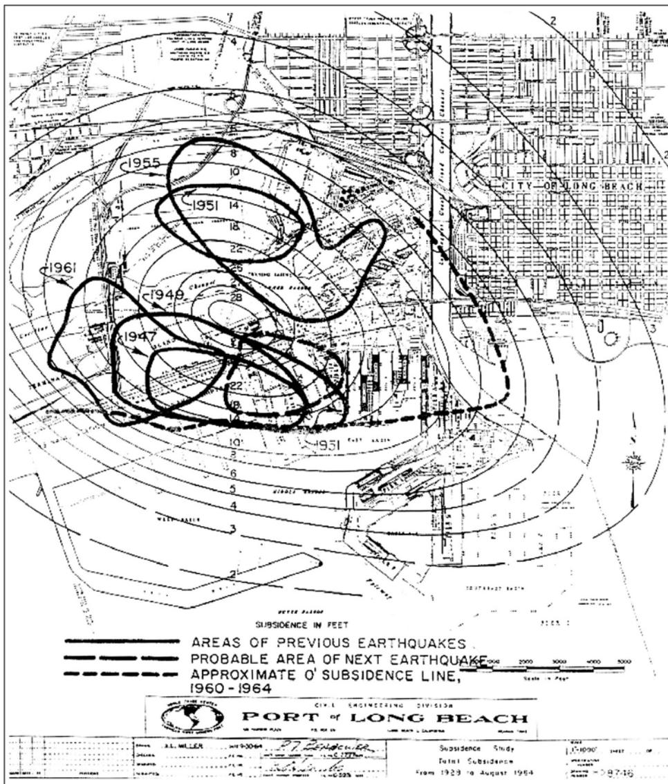
Fig. 13—Subsidence contours and shear areas in Wilmington field, Long Beach, California.
