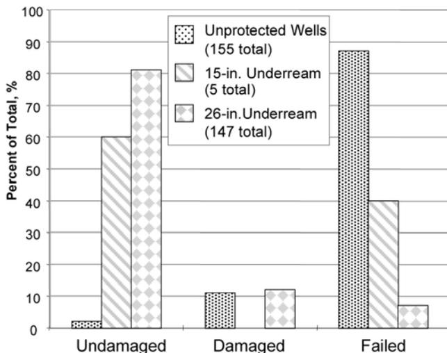
Fig. 12—UPRC well damage in Wilmington field during 4 April 1961 shallow earthquake.
