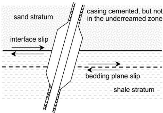
Fig. 10—Underreaming to reduce dogleg rate.
