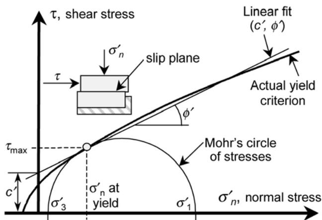
**Fig. 2—Mohr-Coulomb criterion and stresses.**
