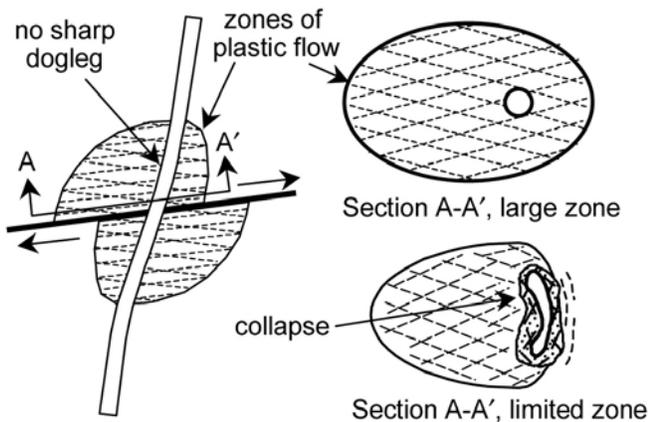
Fig. 17—Plastic formation flow around casing.
