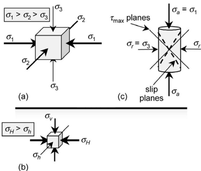
**Fig. 1—Basic stress conditions: (a) principal stress; (b) in-situ stress; (c) triaxial stress.**
