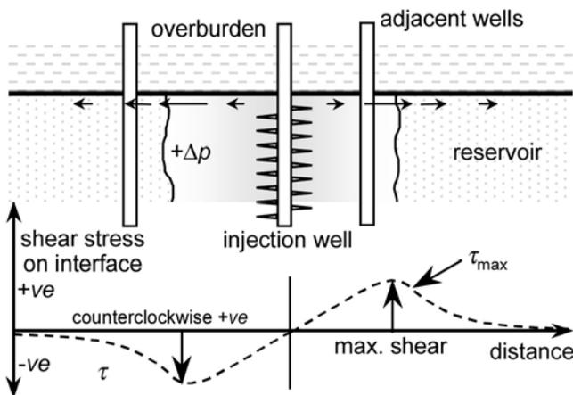
Fig. 6—Injection-induced interface shear stress.
