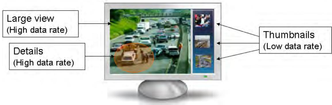
In Figure 3.4 sources V1 and V4 are displayed as thumbnails on viewers M1-M4 only. As such their uplink data rates are 64Kbps, whereas V2 and V3 are viewed in expanded mode so they are uplinked at the HiRes data rates.
