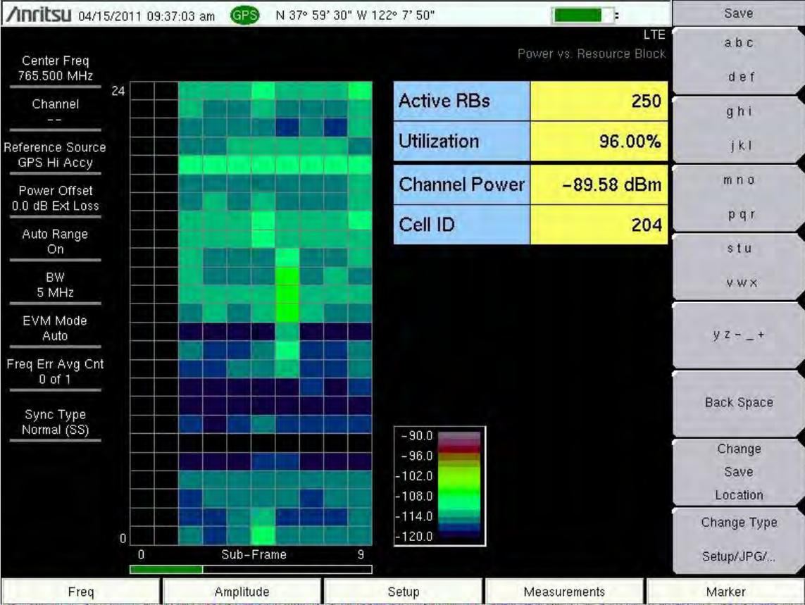
Diagram 3: Edge of cell, 96% system utilization
