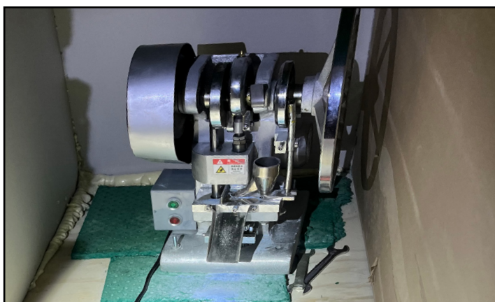
Automatic pill presses can produce thousands of counterfeit pills in a short amount of time. A variety of molds are used to create different shaped pills.
