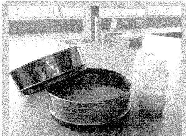
Photograph 2 A small portion of treatment plant post-treatment effluent is sieved at the facility and sent to SUNY Fredonia for analysis.
