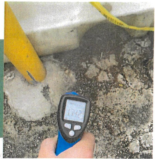
Steam temperature recorded at nearly 180 degrees Fahrenheit in front of 1223 FDR Dr.
