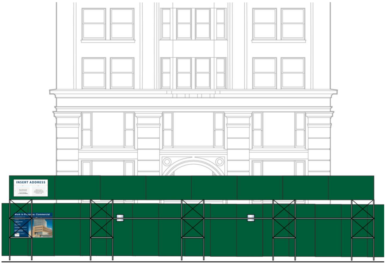
FIGURE 3301.9.2.2 PANEL POSTING ELEVATION DIAGRAM
