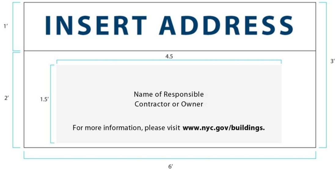
FIGURE 3301.9.2.1(1) SIDEWALK SHED PARAPET PANEL LAYOUT
