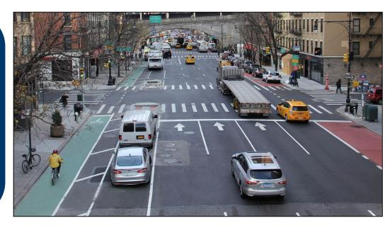
Traffic signals are coordinated to efficiently move vehicles, pedestrians, and cyclists. To best coordinate signals, adjacent intersections have the same signal cycle length, typically 60, 90, or 120 seconds. Each traffic movement is allotted a certain percentage of time in the cycle, known as a phase, based on the number of vehicles, pedestrians, and cyclists moving in each direction.
